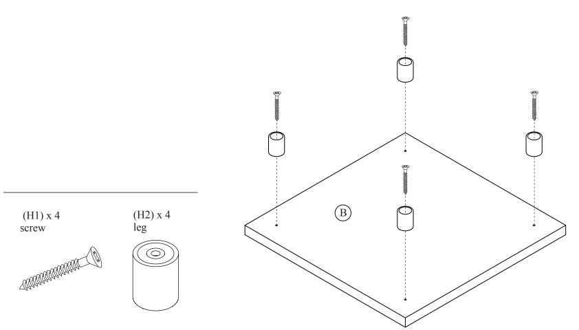
Locate the pilot holes in Panel B and then use a Philips screw driver to install the legs.
