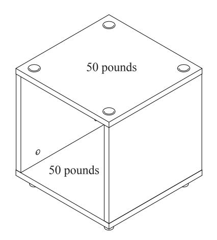
Do not exceed the recommended weight limits on the designated panels. Exceeding these limits could cause sagging, possibly resulting in failure of the panel or bodily injury.
