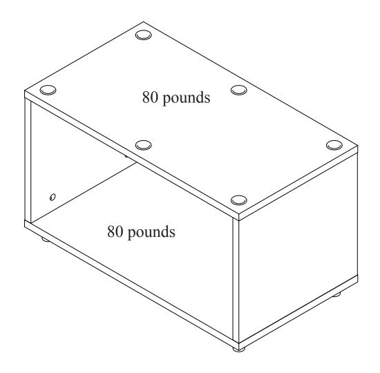
Do not exceed the recommended weight limits on the designated panels. Exceeding these limits could cause sagging, possibly resulting in failure of the panel or bodily injury.
