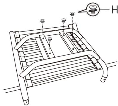
**IMPORTANT NOTE:** Screws and washers (Parts H) are preassembled into the underside of the seat (Part B). Remove screws and washers from seat and then use to attach Part C to Part B, as shown in step 1.
