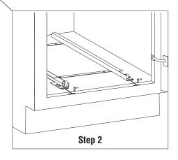
Position front of mounting frame 2" (50mm) from front edge of cabinet. Then mark each hole on mounting frame with pencil.
