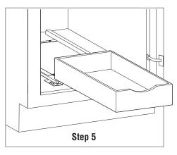
Insert Roll-Out Drawer using guide rails on mounting frame that is now attached to the bottom of the cabinet.
