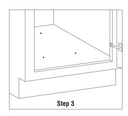
Remove mounting frame to reveal marked hole locations, use drill with 1/16" drill bit to create pilot holes for screws (4 holes in total)
