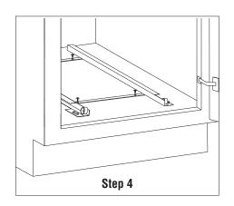
Use mounting screws (4 in total), to secure mounting frame to bottom of cabinet.
