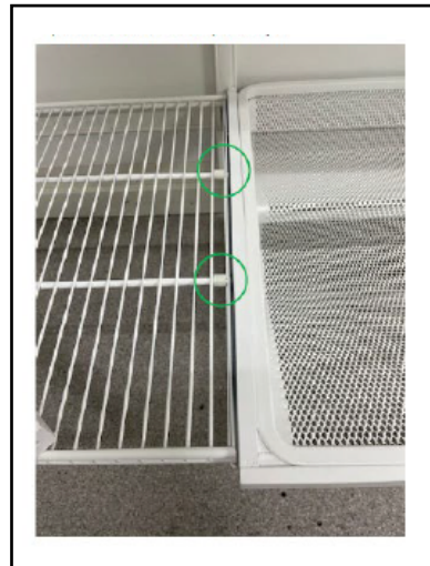
Wire Shelf in correct and secured position with C-Clips in place.
