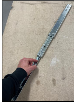
Push down on the black plastic part and remove the inner Drawer Slide.
