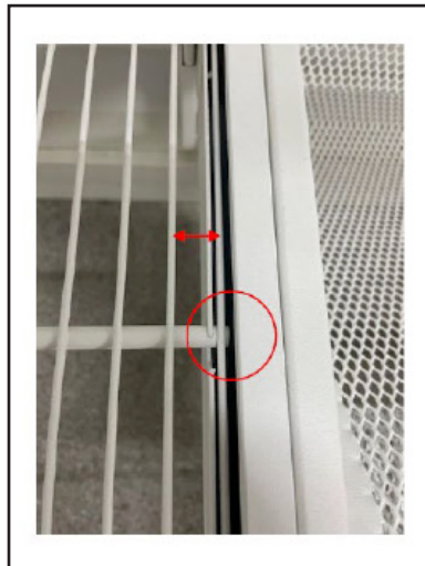
Close-up showing gap caused by movement of the Wire Shelf and Wire Outstick.
