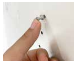
Double Dowels (#7) inserted in Partition
