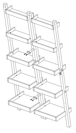
1. Locate pilot holes on the backs of the legs.
