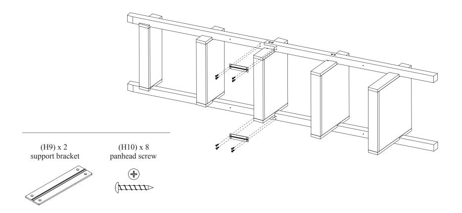
Locate pilot holes on the backs of the legs.
