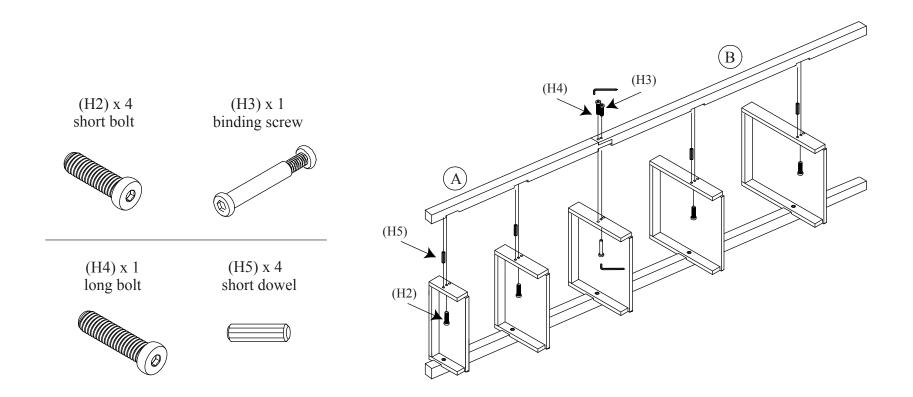
1. Fasten right leg assembly [AB] to Third Shelf [G] using a long bolt and binding screw.
