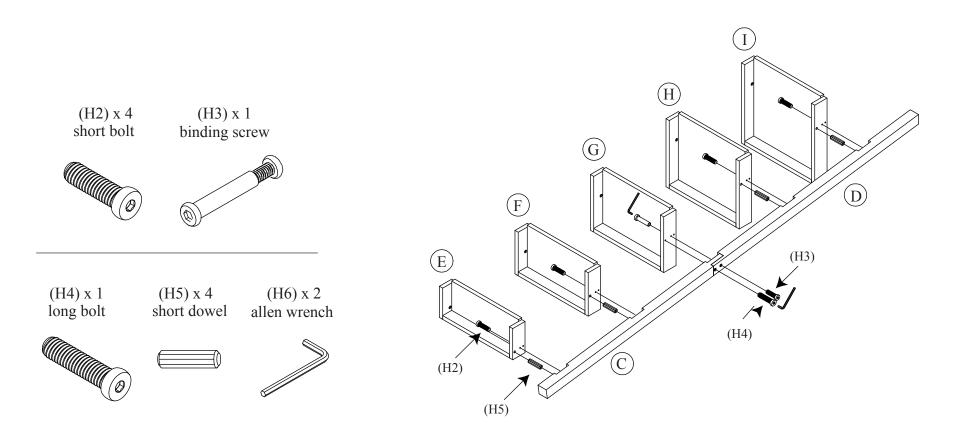
1. Fasten Third Shelf [G] to the Leg Assembly [CD] using a long bolt and a binding screw.
