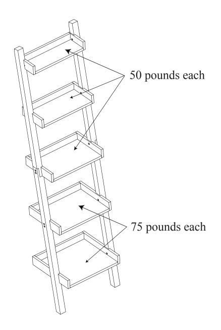
Do not exceed the recommended weight limits on the designated panels. Exceeding these limits could cause sagging, possibly resulting in failure of the panel or bodily injury.
