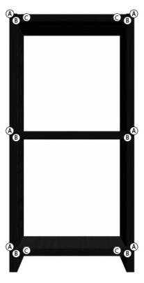
**Step 3**: Use a Phillips screwdriver to screw in and tighten a Bracket (C) using 2 Bracket Screws (D) at four corners of the unit.
